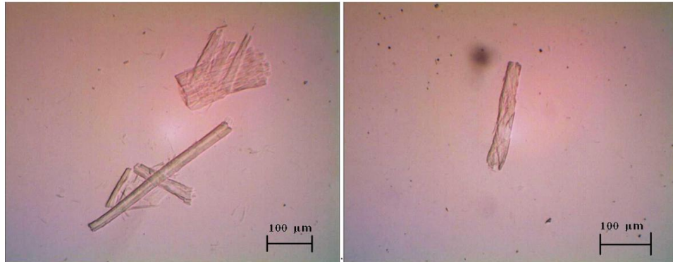
Fig. 2. Optical micrograph of cellulose extracted using \text{NH}_3 neutralization, before centrifugation
