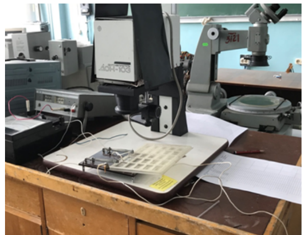
Fig. 1 Stand for measuring the current-voltage characteristic.
