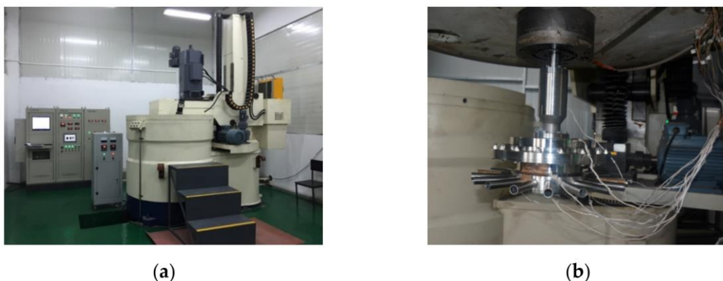
Figure 10. Test equipment: (a) The rotor high-speed rotating tester; (b) Installation schematic.
