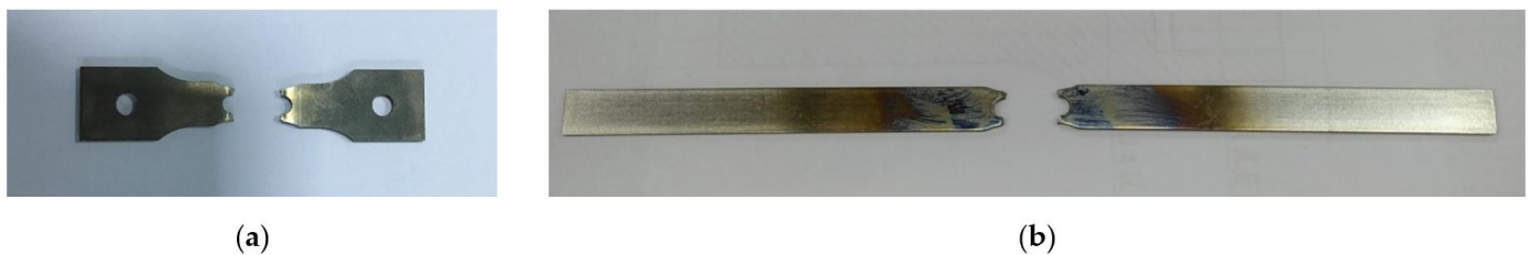
Figure 19. The fracture of the specimens after testing: (a) Clamped by pin holes; (b) Clamped by hydraulic pressure.
