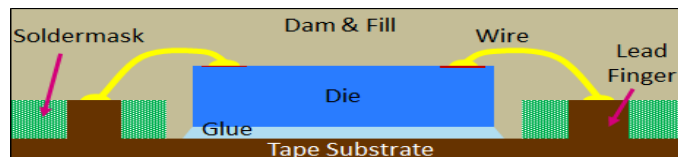
Fig. 4. Substrate design improvement with augmented lead finger configuration
