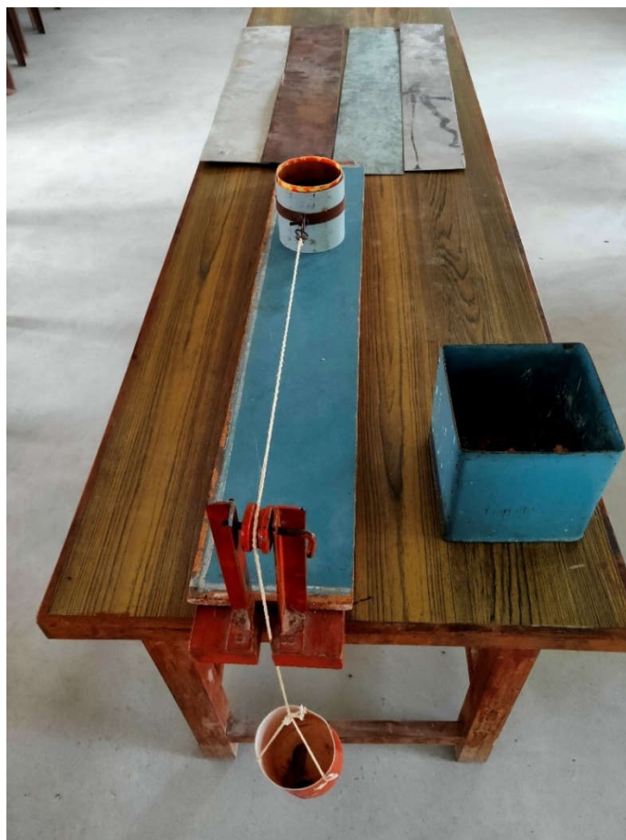
Plate 1. Apparatus for measuring coefficient of static friction
