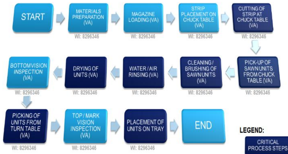
Fig. 5. Package singulation: A detailed process flow
