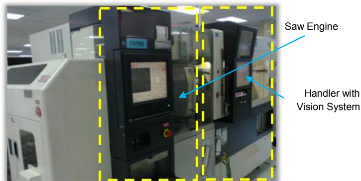
Fig. 2. Package singulation machine with integrated handler and vision system
