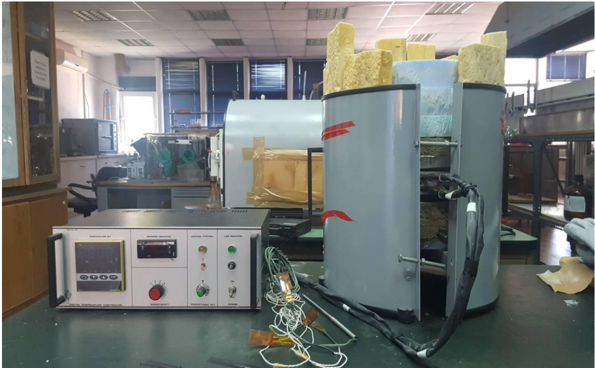
Fig. 2. Thermal conductivity measurement apparatus
