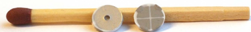
Figure 10. Two microthrusters leaning against a normal match. Left one shows top side containing gas inlet hole and right one shows the electrical connector pads on the bottom side.
