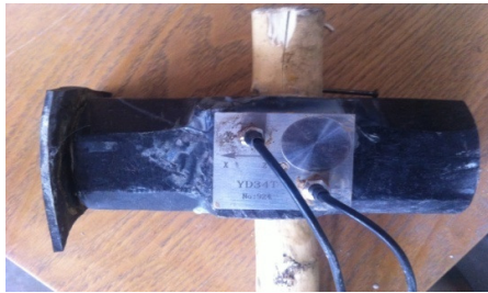
Fig. 4. Heavy hammer under test fixed-point vibrating
