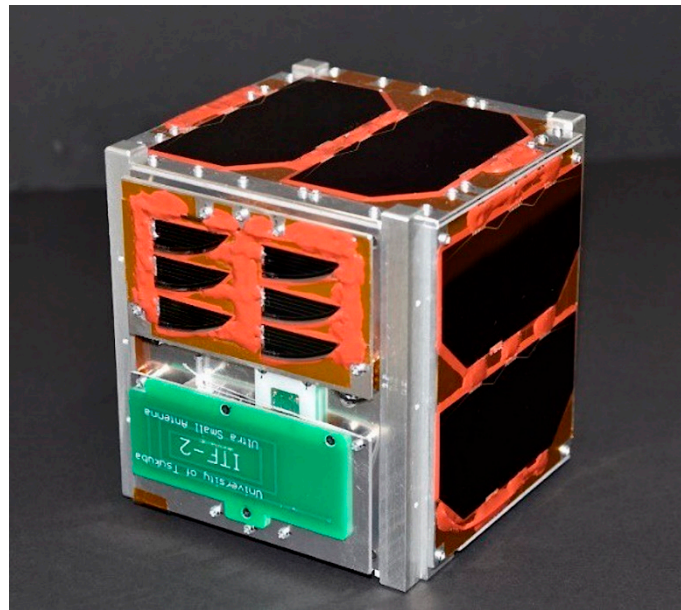
Figure 1. University of Tsukuba CubeSat ITF-2 (YUI-2).
