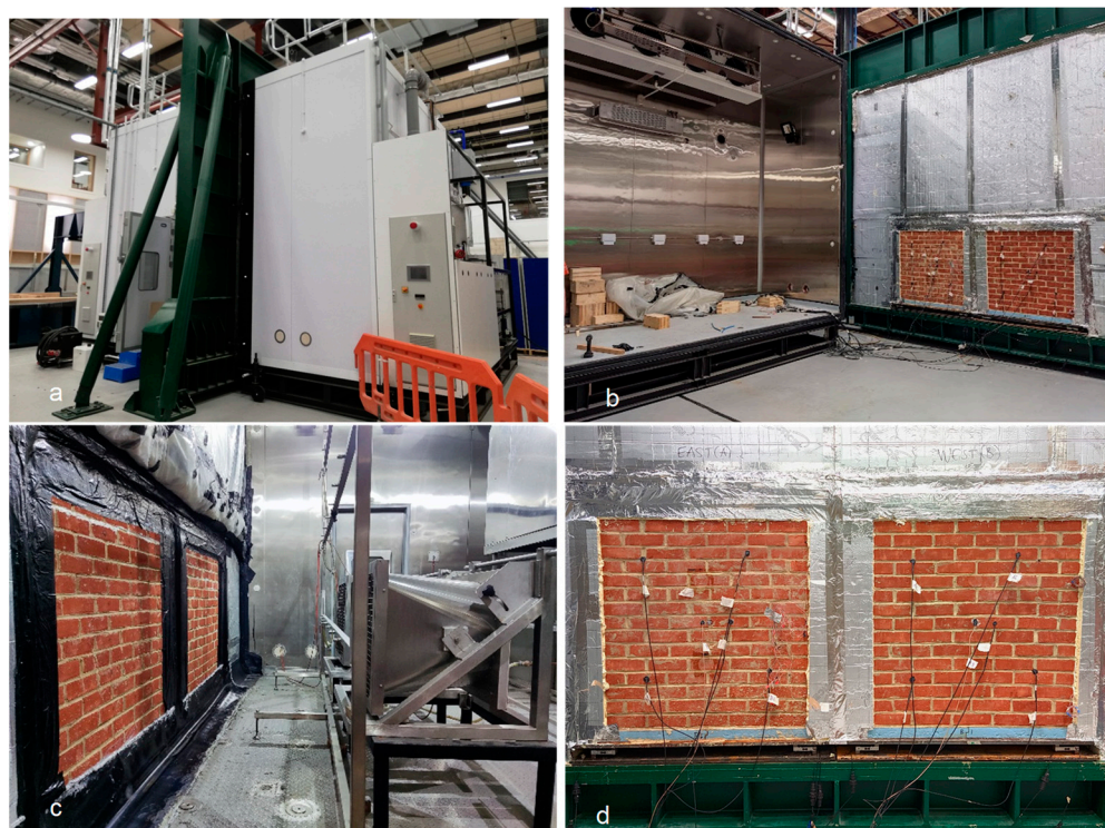
Figure 3. Outdoor–indoor-coupled environmental chambers at UCL-StrEnTHE laboratory (Strength and Environmental Testing @ Here East) and wall specimens: (a) overview of the environmental chambers and loading rig; (b) open view of the mobile indoor chamber and specimens; (c) WDR equipment in the outdoor chamber; (d) view from indoor chamber of wall specimens mounted on loadcells and equipped with T&RH sensors.
