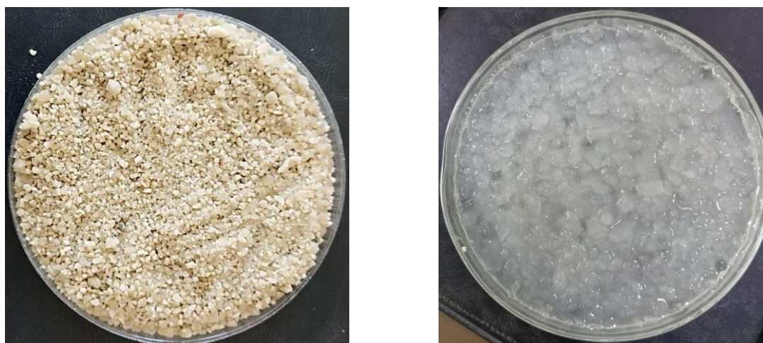
Fig. 1. Hydrogel polymer before and after water absorption
