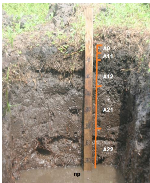
Fig. 4. Shades of 0 - 75 cm layers and water table of the lowland soil
